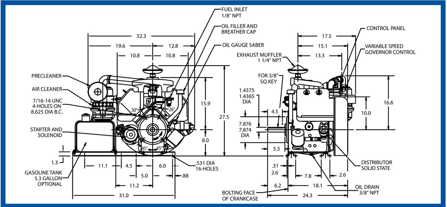
\* Net Weight Dry Standard Engine 530 lbs. (240 kg)
