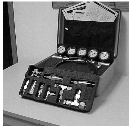
Figure 3-2 Hydraulic Pressure Diagnostic Test Kit
