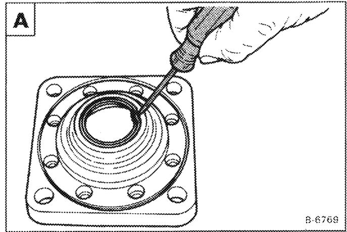
Remove the shaft seal and brass back-up ring **B**.
