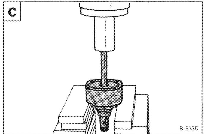
Remove the seal from the bearing housing **D**.
