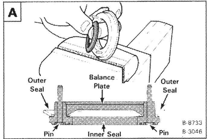
Remove the outer seal from the balance plate **B**.
