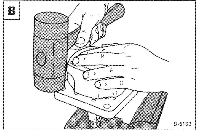
Use a press, remove the shaft and bearing assembly **C**.
