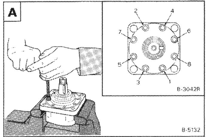
Remove the mounting flange from the housing **B**.
