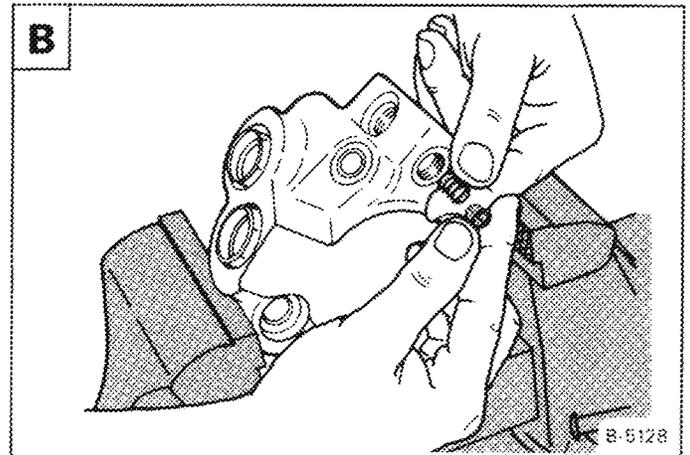
Use a punch, remove the poppet, spring, O-ring, shuttle and plug **C**.
