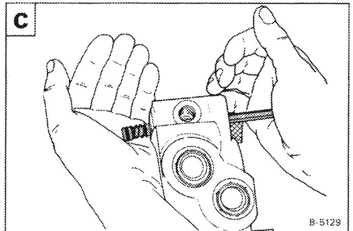
Remove the two springs from the balance plate **D**.
