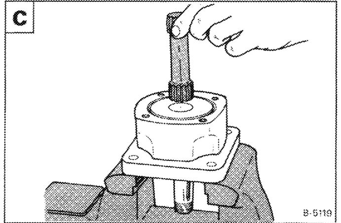
Remove the O-rings (large and small) from the bearing housing **D**.
