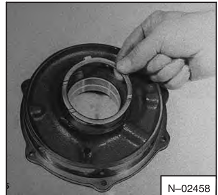
Fig. 7A-114 Installing Thrust Washer
