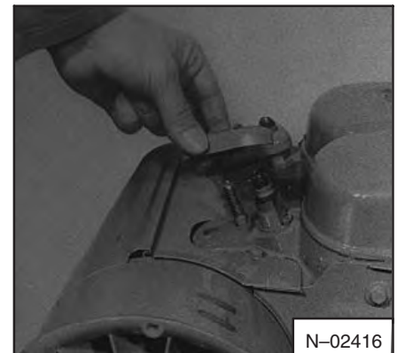
Fig. 7A-23 Removing The Yoke
