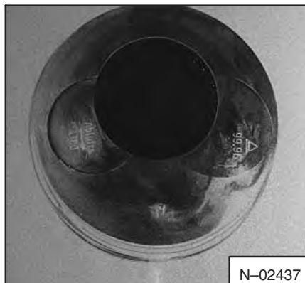
Fig. 7A-83 Arrow On Piston
