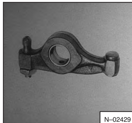
Fig. 7A-65 Checking Bushings
