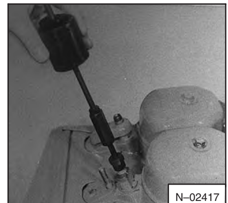
Fig. 7A-24 Removing The Injector
