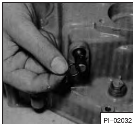
Fig. 7A-99 Installing O-Rings On Shaft
