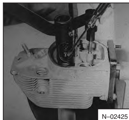
Fig. 7A-55 Removing The Valve Springs
