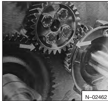
Fig. 7A-119 Aligning Timing Marks
