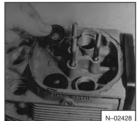
Fig. 7A-64 Installing Spring Caps
