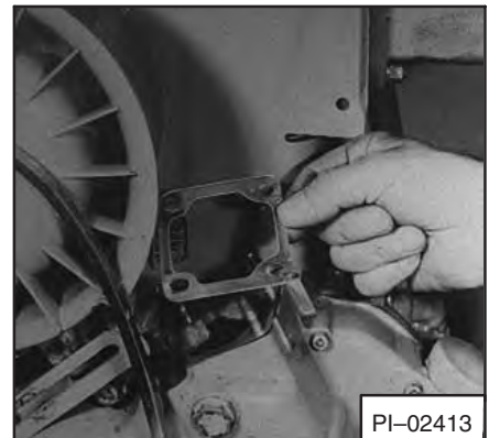
Fig. 7A-12 Adding And Removing shims
