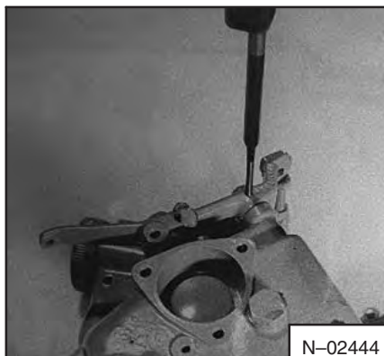
Fig. 7A-93 Removing Pin
