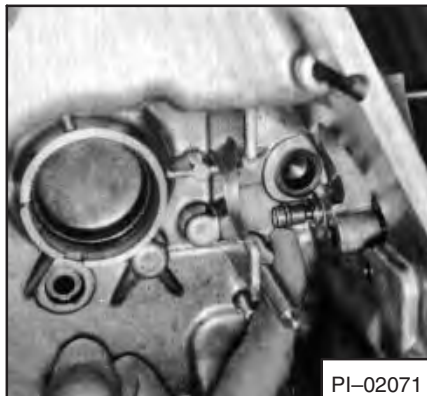
Fig. 7A-91 Lubrication Of O-Ring
