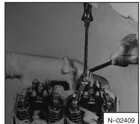
Fig. 7A-72 Adjusting Rocker Arms
