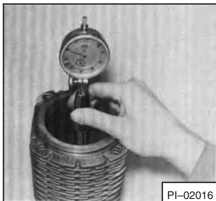
Fig. 7A-79 Checking The Cylinder Wall
