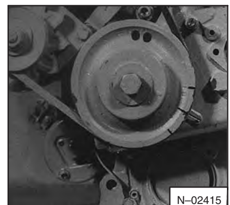
Fig. 7A-17 Marking Half-Way Position
