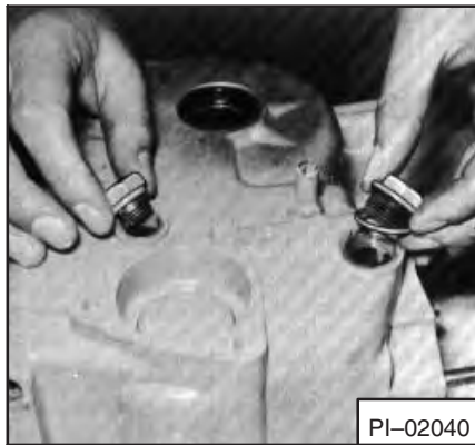
Fig. 7A-88 O-Rings On Plugs
