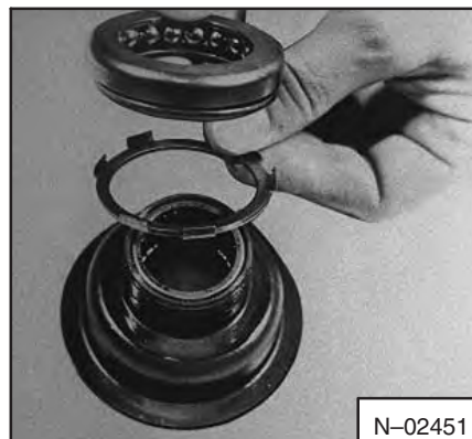
Fig. 7A-105 Installing Shims
