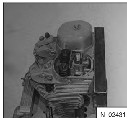
Fig. 7A-67 Checking Alignment Of Heads
