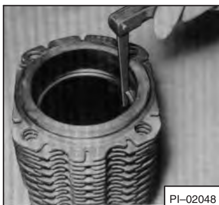
Fig. 7A-81 Checking The Ring Gap
