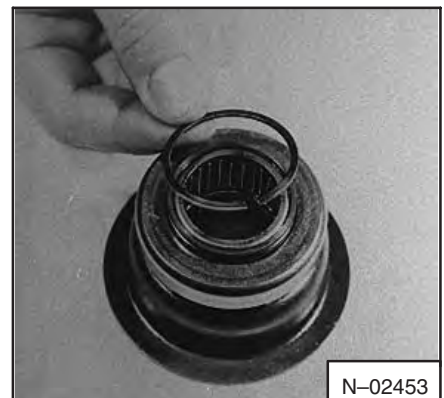
Fig. 7A-106 Retainer Ring
