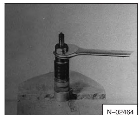
Fig. 7A-25 Disassembly Of Injection Nozzle
