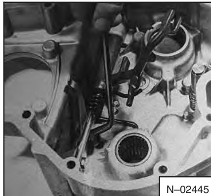
Fig. 7A-97 Installing Governor Spring
