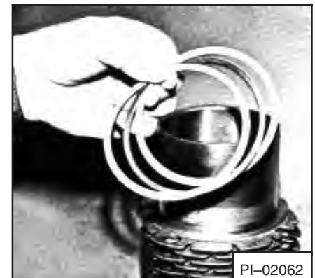
Fig. 7A-34 Installing Shims
