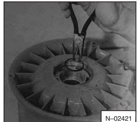
Fig. 7A-31 Removing The Snap Ring
