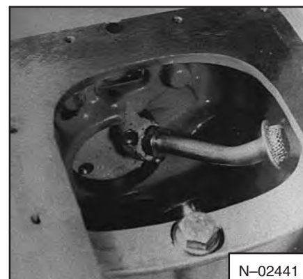
Fig. 7A-86 Removing The Oil Pump
