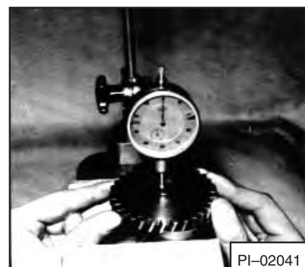
Fig. 7A-87 Checking End Play Of Oil Pump
