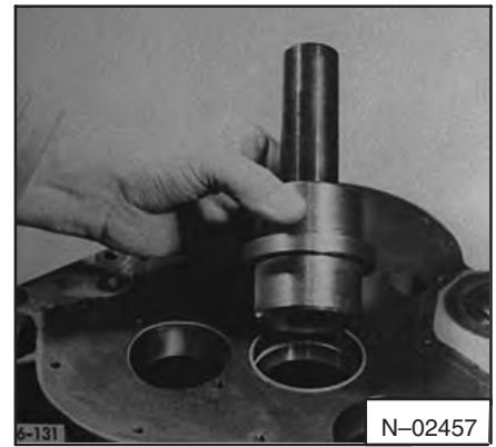
Fig. 7A-109 Installing Camshaft Bearings
