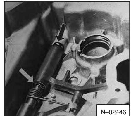
Fig. 7A-98 Installing Snap Rings
