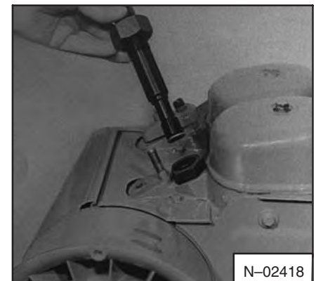
Fig. 7A-33 Checking Compression
