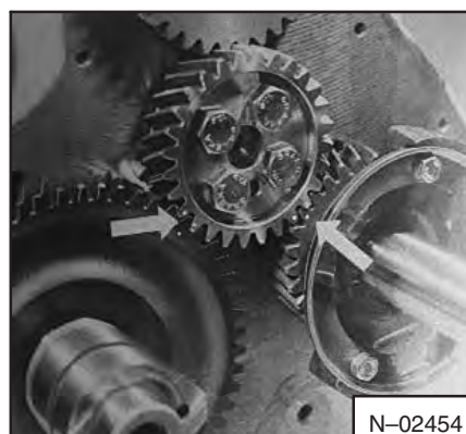
Fig. 7A-107 Alignment Of Gears
