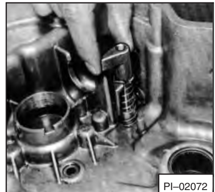
Fig. 7A-92 Setting Spring Tension
