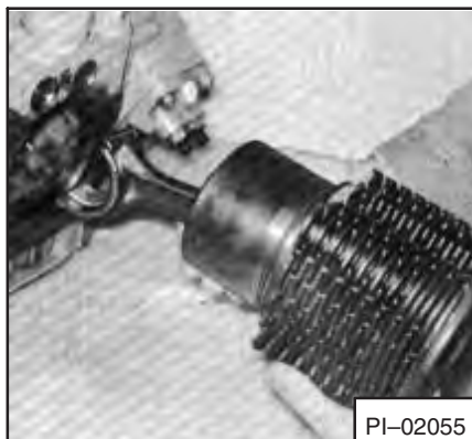
Fig. 7A-75 Removing Rod And Cylinder
