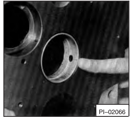
Fig. 7A-113 Installing Bearing
