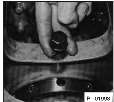
Fig. 7A-116 Installing Crankshaft
