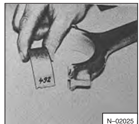
Fig. 7A-74 Marking Bearings
