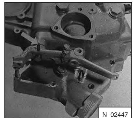
Fig. 7A-100 Installing Roll Pins
